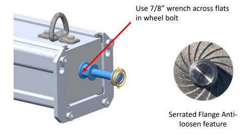
Tighten the wheel bolt firmly using a 7/8" wrench. There is an anti loosen feature on the face of the wheel bolt which will help the bolt stay seated, so it does not need to be extremely tight. Repeat for both sides
