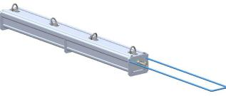
Step5b: Pull the handle out until it bottoms out on the quick clean off flange.
