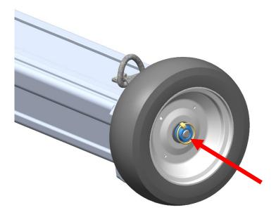
Re-install the retainer and the 3/16" lynch pin. The holes in the retainer and wheel bolt should be aligned. Note: There is a bit of lateral play in the wheel when installed, this was designed this way for optimum rolling behaviour. Repeat for both sides.
