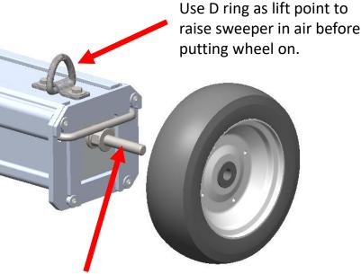
Install the flat proof wheel on the wheel bolt. Note the orientation of the wheel as shown. The bump wheels will not work as intended if the wheel is installed the other way around. Repeat for both sides.
