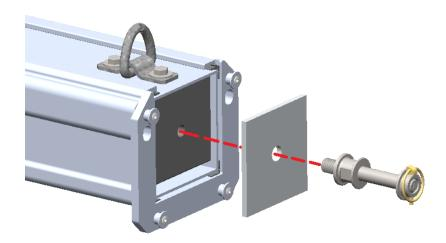
Thread the stainless-steel wheel bolt through the hole in the aluminum end cap and then hand thread the wheel bolt into the end cap of the magnet assembly. There is only one way the end cap can go in, so if it is tight you will need to turn it 90 degrees and try again. Repeat for both sides.
